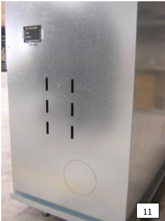
Cut-out opening – connection of ambient air
